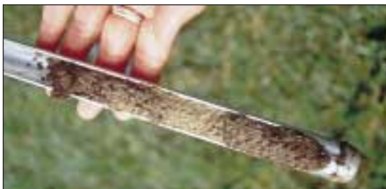
An example of a core-extracting soil probe.
