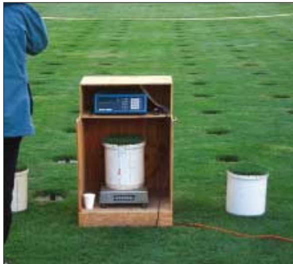
The mini-lysimeter gauges water use under actual turf conditions. This photo at Washington State University’s research site in Puyallup, shows mini-lysimeters being weighed. The pots are weighed for daily water evaporation, rewetted and returned to their “holes” in the turf. These scientific measurements under controlled procedures help researchers better understand low-water use.
