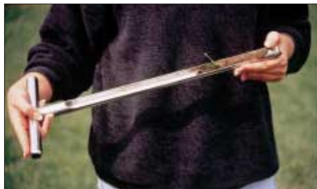
Using a soil probe for observing and feeling the soil for moistness.
