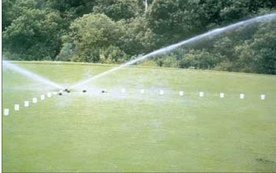
Catch cans determine irrigation distribution uniformity, after which adjustments will be made to improve uniformity and save water.
